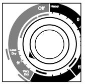
Depending on your model, the Automatic cycle uses either an electronic or automatic DRY-MISER® control that senses the moisture in the load and shuts off the dryer when the selected dryness is reached. The Cycle Control knob
