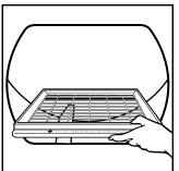
door opening. Push down to secure rack on frame.
