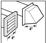
3. You can exhaust from the rear, left, right, or bottom of the dryer.
